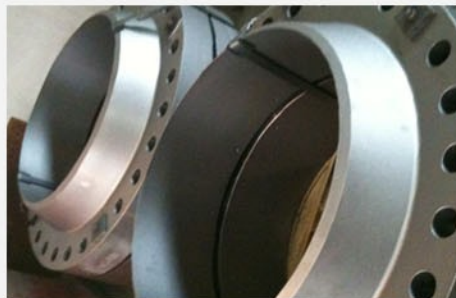
WN RF 30" 600# B16.47/A - ASTM A694 F65 SAND BLASTED
